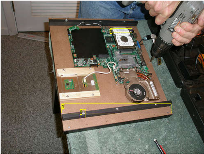
Image Notes 1. Spray-painted Black to hide laptop's guts. 2. Where the picture wire will be attached to it 3. Hard Drive Zip-Tied Down
